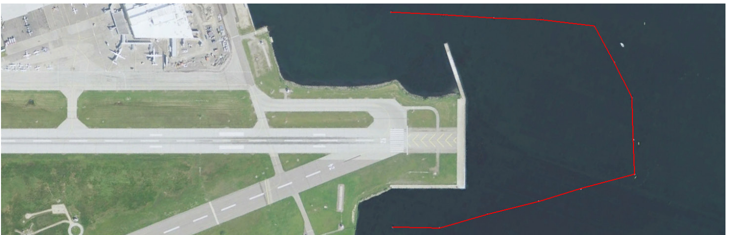
Runway 26 - 1,216 meters in length. No runway approach lighting system. Red is current MEZ
