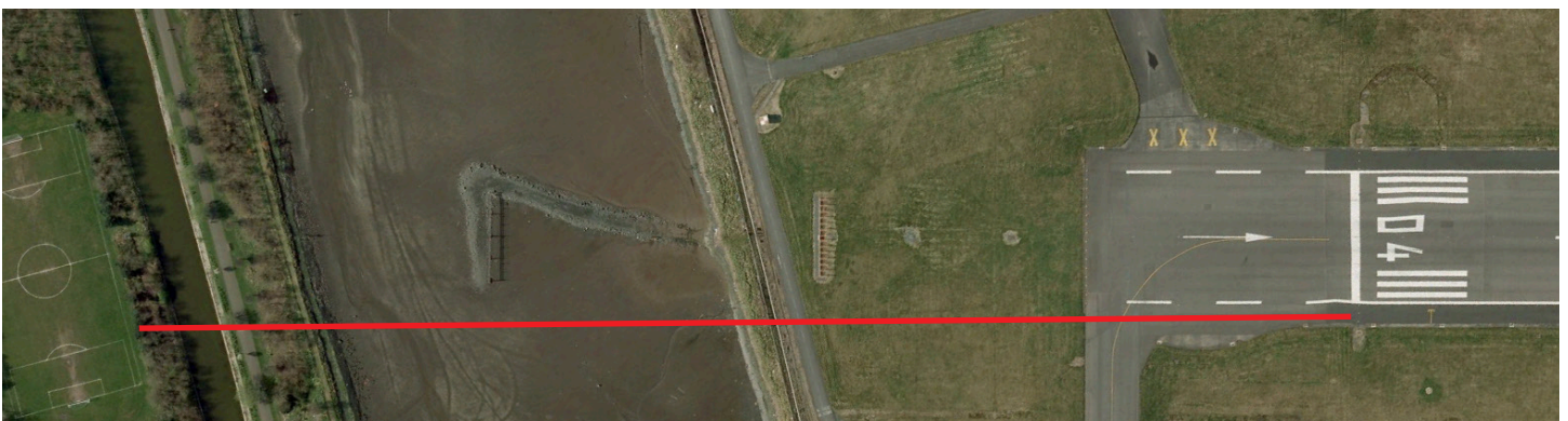
Runway 04 - 1,829 meters in length. 04 has land based approach lighting to a distance of 440 meters from the threshold.
